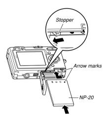
• Push the bottom of the battery, and make sure that the stopper securely locks the battery in place.
